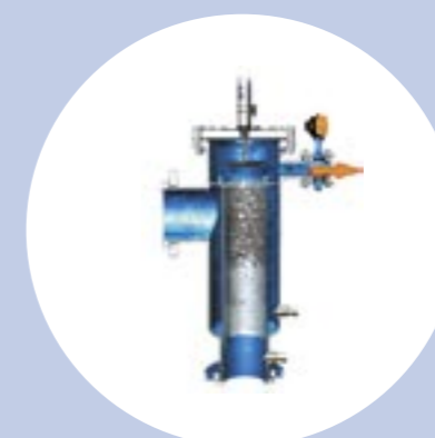
Flushing phase one Cleaning is initiated by a timer or differential pressure control. The flushing valve opens and large particles are flushed out.
