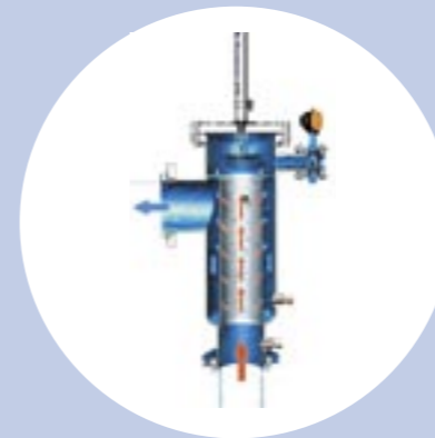
Normal filtering operation The flushing valve is closed. The piston remains outside the strainer basket.
